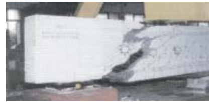
Fig. 13 Prestressed Beam-Failure by Web Crushing
