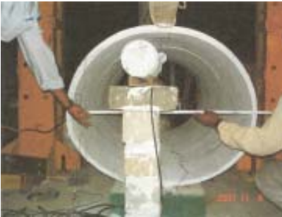
Fig. 21 Deformability of SIFCON Pipe
